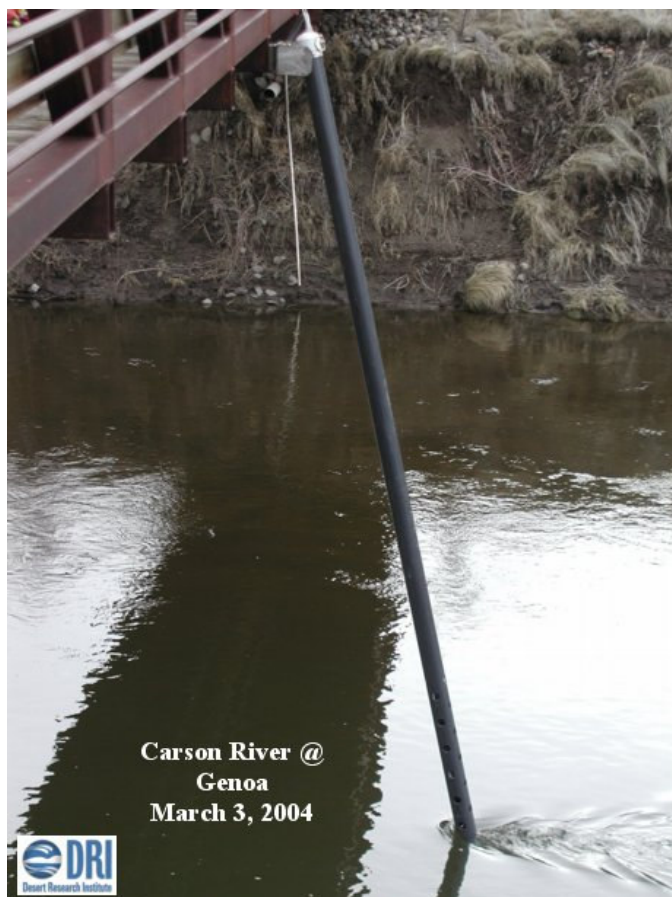
Figure 4. Turbidity Sonde Deployment by Desert Research Institute – Carson River at Genoa Lakes Golf Course (Photograph by R. Susfalk, 2004)
